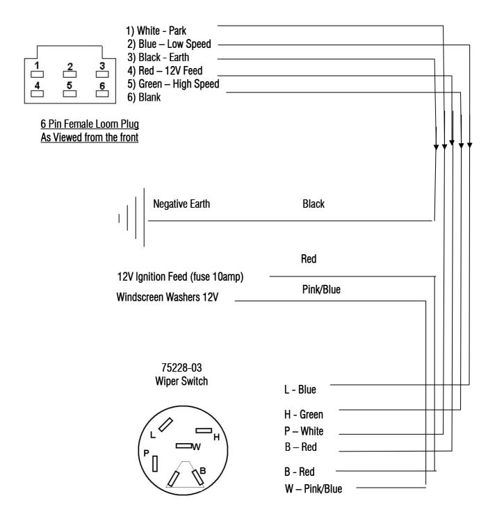
Wiper switch system is 12V Positive Feed
